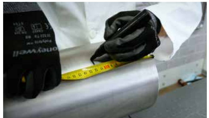
Figure 15 - Marking the insertion depth
