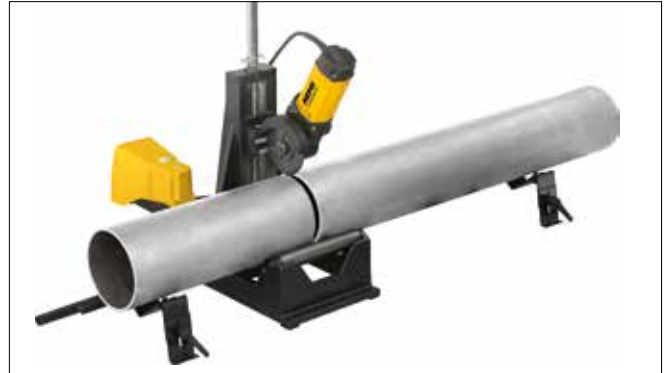
Figure 12 - Cutting the pipe to length
