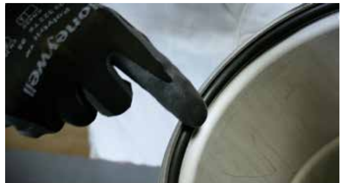
Figure 16 -Checking the sealing ring
